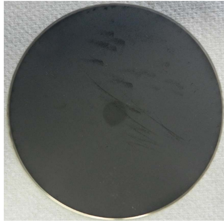
O 2 electrode side, dismantled cell
